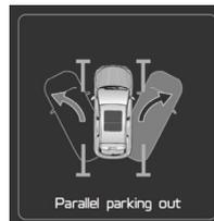
3. Select pulling-out direction by activate turn signal light lever (to left or right).
