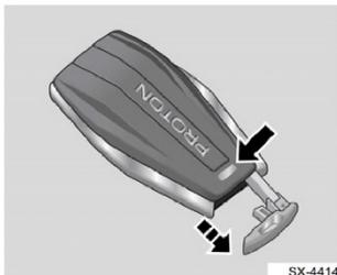
Press the release button on the back of the intelligent key, then you can pull the mechanical key out.
