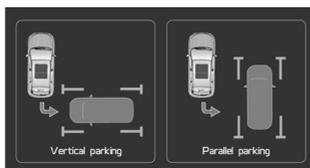
4. Activate right or left turn signal to find parking slot at the corresponding side. Display will show the available parking slot.
