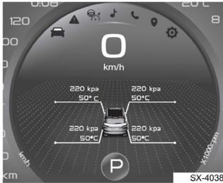
The information of pressure and temperature of the tyre can be fed back to the meter instrument via the tyre pressure sensor and displayed in real time on the meter instrument. The tyre temperature display is accurate to 1 °C and the tyre pressure display is accurate to 1 kPa.
