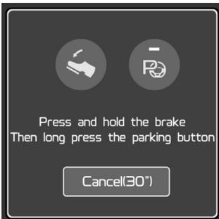
6. Release brake pedal to start parking out / pulling-out the vehicle.
