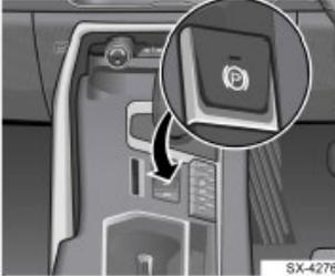
The electric parking brake switch button is behind the gear lever.
