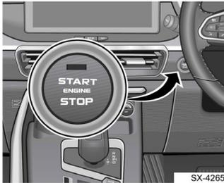
This vehicle is equipped with a push-button ignition switch. To operate the system, the intelligent key must be inside the vehicle and is detected.
