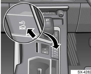
During the drive on downhill road, the downhill speed can be controlled with the accelerator pedal or brake pedal is pressed.
